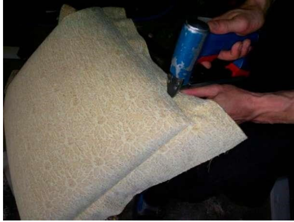
Picture 4.9: Hammering of stuffing material
