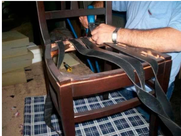
Picture 4.4: Hammering colons on the lining or without lining to stable furniture frame
