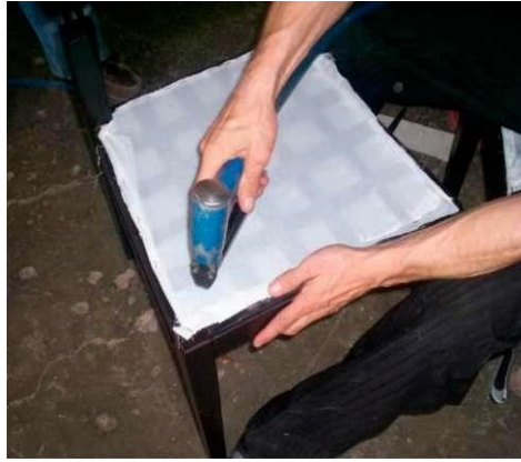
Picture 4.6: Hammering of lining cloths
