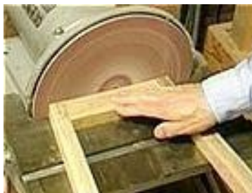
Picture 1.9: Picking up excesses on the sanding machine
