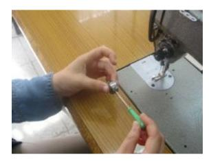
Picture 3.12. Shuttle screw tightness or slack adjustment
