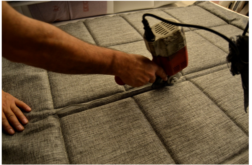
Picture 2.5. Quilting cut with round blade cutting engine
