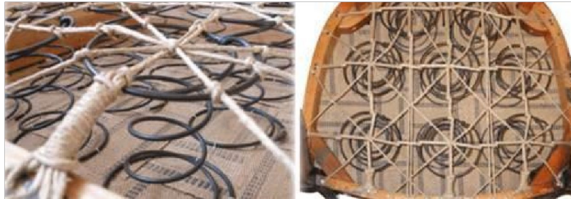
Picture 6.9: The surface of spirial arched upholstery
