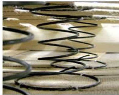
Picture 6.8: Binding of spirial arches on furniture frame
