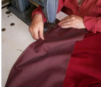
Picture 6.20: Sewing face cloth in machine
