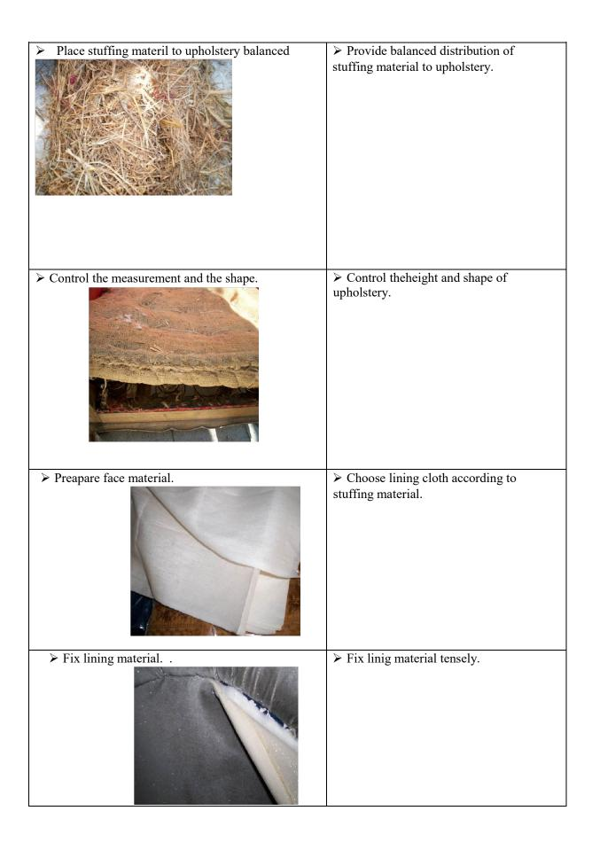
> Prepare fiber. . > Cut fiber according to furniture frame. > Attach fiber by placing. > Attach fiber straightly and firmly. > Prepare face fabric. > Cut lining cloth by leaving necessary extras of fabric . > Attach fabric tensely. Fix with staples and nails. ➤ Clean fabric'extras with utility knife or > Clean fabric'extras by cutting. scissors.
