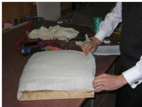
Picture 5.16: Binding of quilted front part
