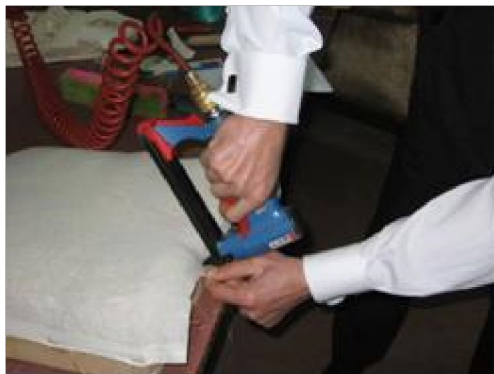
Picture 5.18: Ending of sparse quilted connection
