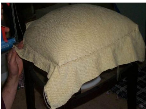
Picture 5.21: Stuffing material attached to upholstery
