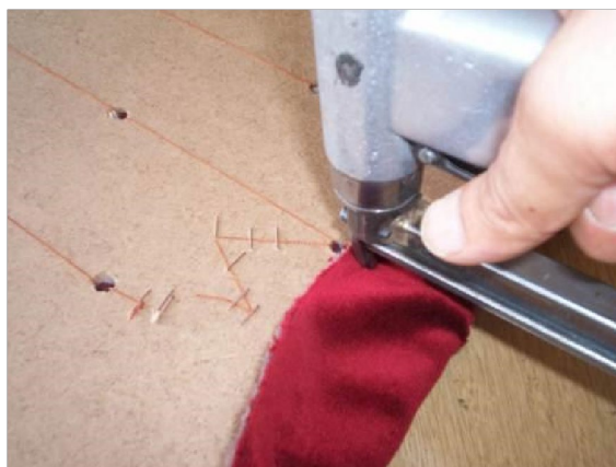
Picture 4.23: Fixing of face cloth
