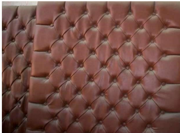
Picture 4.10: Quilted upholstery on the plywood
