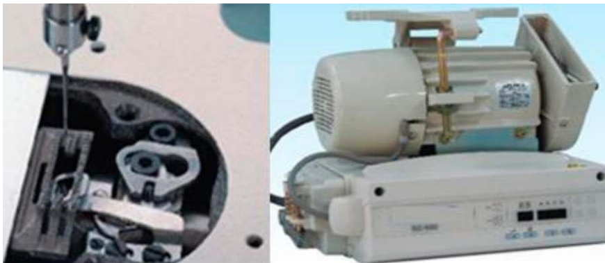
Picture 3.40: System of cutting rope, box of engine and control
