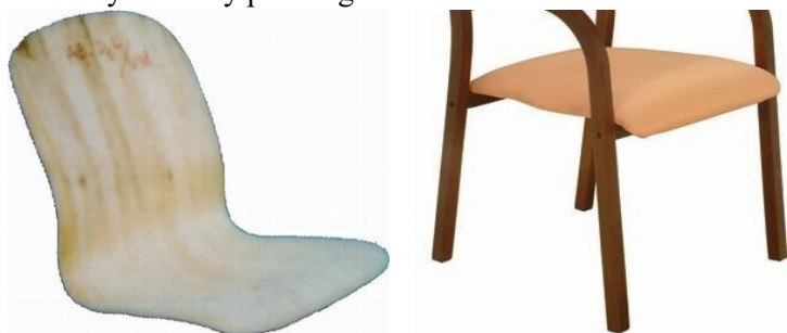
Picture 2.4: Furniture frame with the technic of bending
