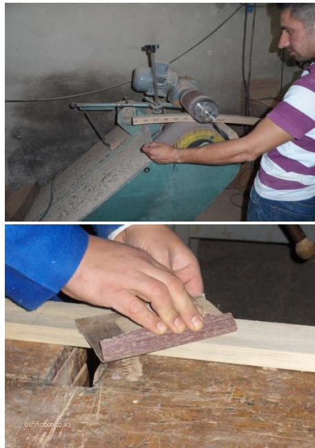
Picture 1.11: Work the surface of the workpiece and rough sanding the machine
