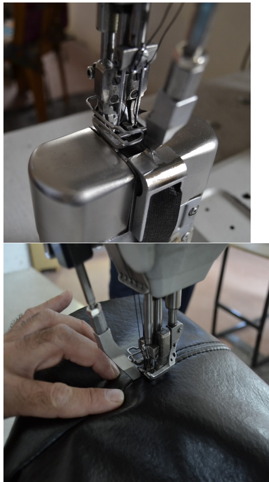
Picture 4.4. Double needle sewing machine needle condition and application
